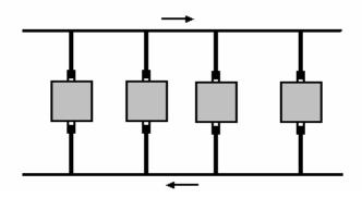
To transmit a cell, a station has to know whether the destination is to the left of it or to its right. If the destination is to the right, the sender uses bus A. Otherwise it uses bus B. Data are inserted onto either bus using a wired-OR-circuit, so failure of a station does not take down the network.
